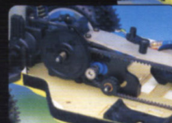
◀ Adjust belt tension using pulley-gear
